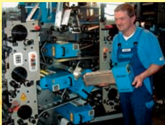
One of PAGO's requirements in the very first system specification was a modular interchangeable UV system.
