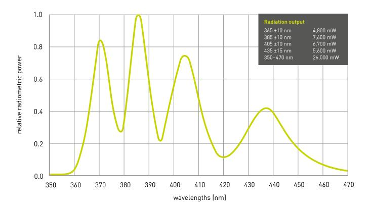
In order to optimize effectiveness in combination with selected photoresists, the spectral output of SPOTcure 09 systems is customizable. A wide range of applications is covered by the standard photolithography con-
